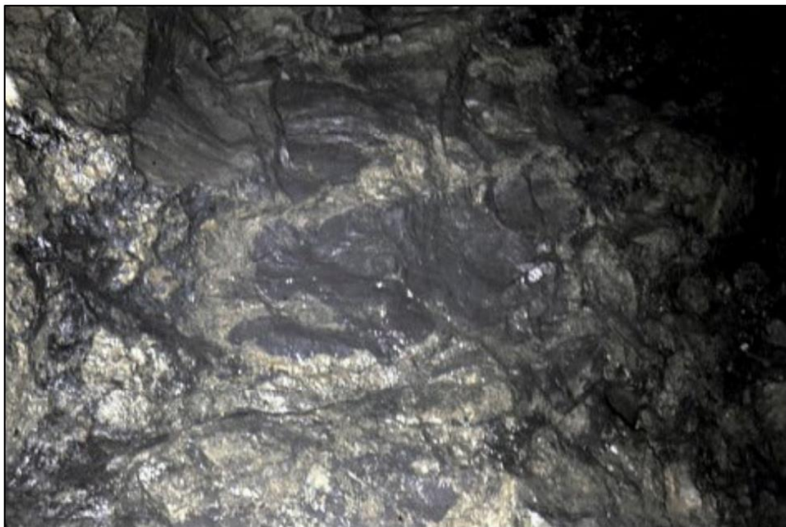
Figure 7-6: Banded and Brecciated Massive Sulphide Mineralization
